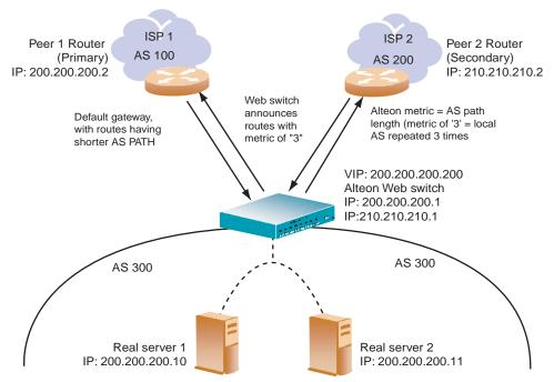
Figure 1-4 BGP Failover Configuration Example
